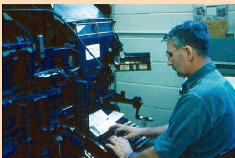
Brother Valerian Tibodeau SDS works on the linotype machine
